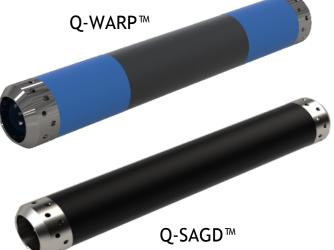
The Q-SAGD<sup>M</sup> was designed for simple onsite slip-on installation onto casing or tubing in SAGD injection wells. The design features a high-temperature (HT) swelling element in combination with Ruma Products' unique slip-on O-ring free design, eliminating the need for bonding agents throughout the swellable packer assembly.
